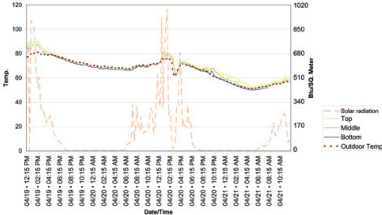
Figure 33.A. Test 6: Sunlight Closed/Air Flow graph.
