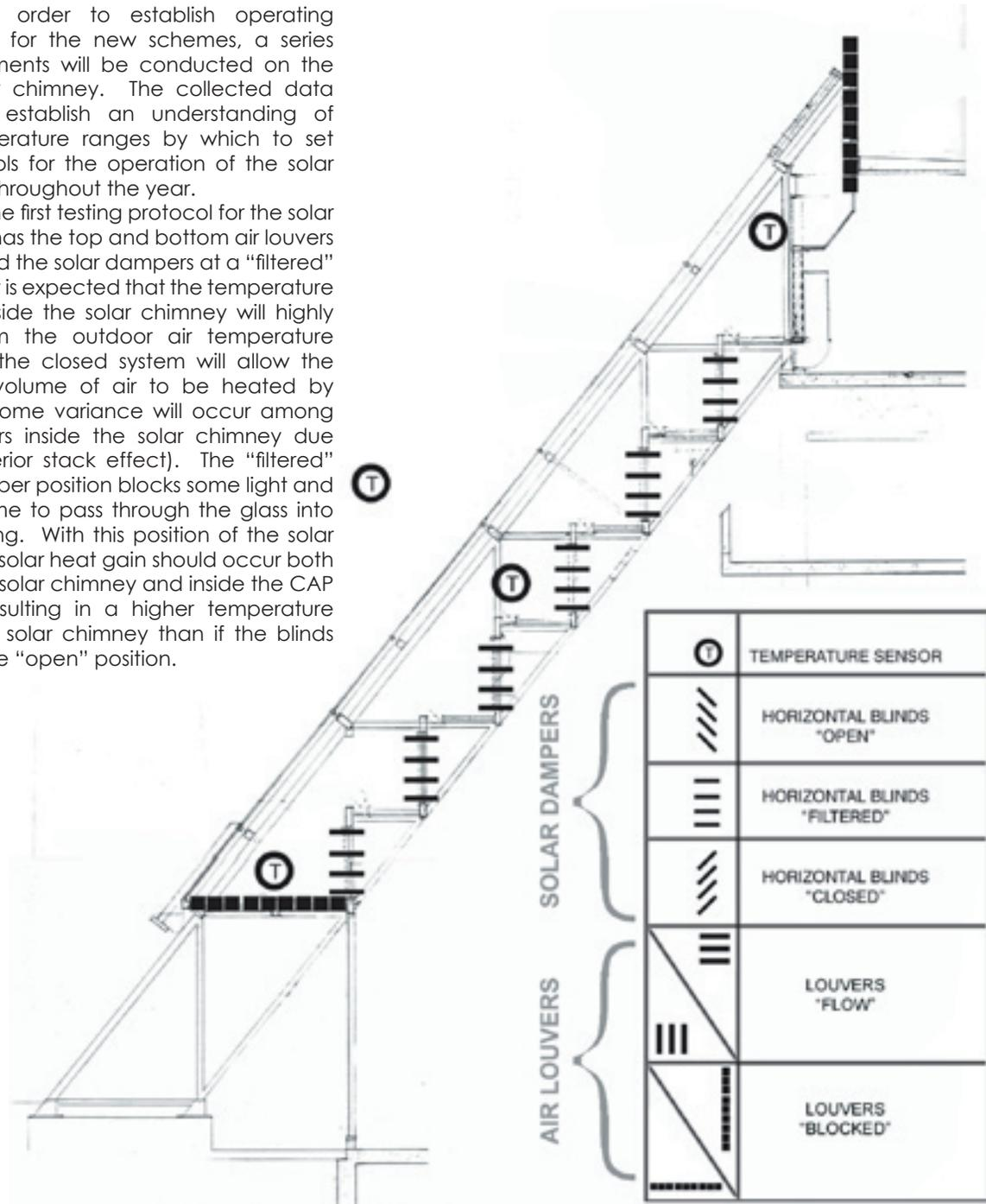
**Figure 18.A.** Test 1: Sunlight Filtered/Air Blocked.
