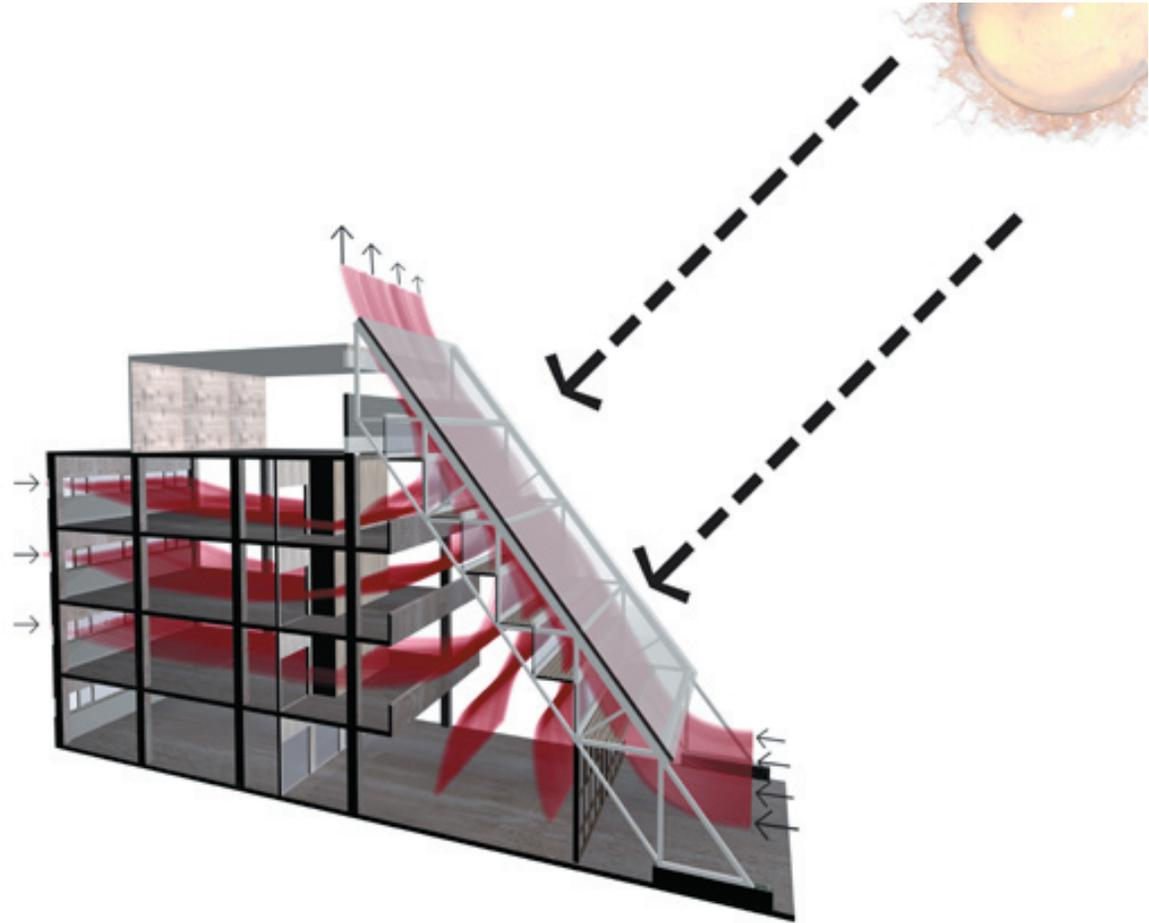
**Figure 14.A.** Natural Ventilation scheme A.
