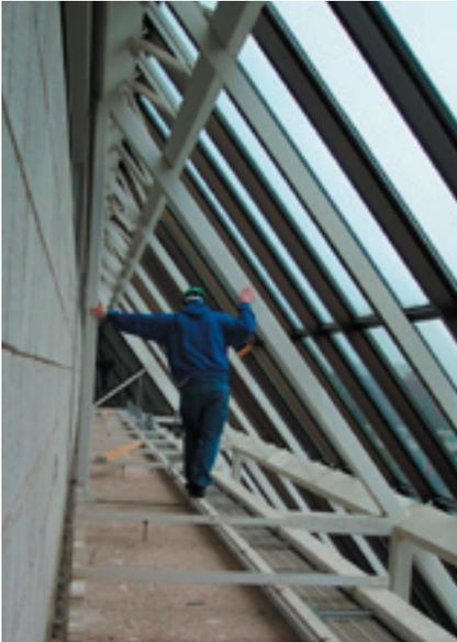
**Figure 24.1.** Balancing on the walkable area to place the temperature recording devices inside the CAP solar chimney.
