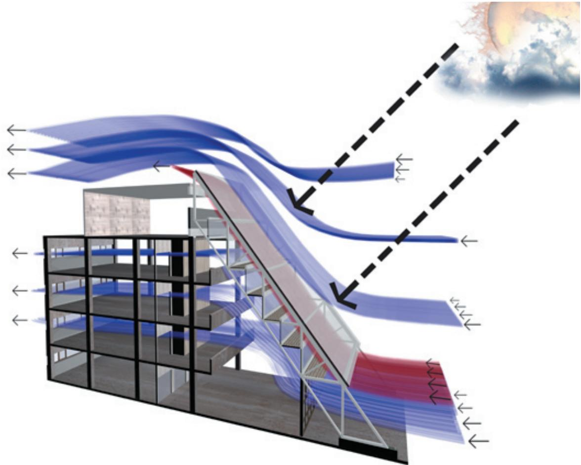
**Figure 16.A.** Natural Ventilation scheme C.
