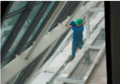
**Figure 24.2.** Placing the StowAway temperature recording instruments inside the CAP solar chimney.
