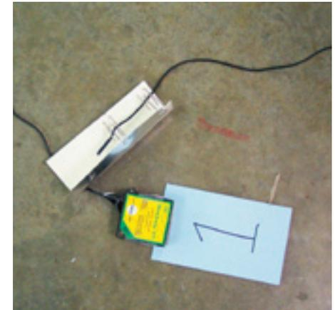
Figure 25.1. StowAway temperature recording device w/wire sensor, sun shield, and label. (Photo by Robert J. Patton, 2003)
