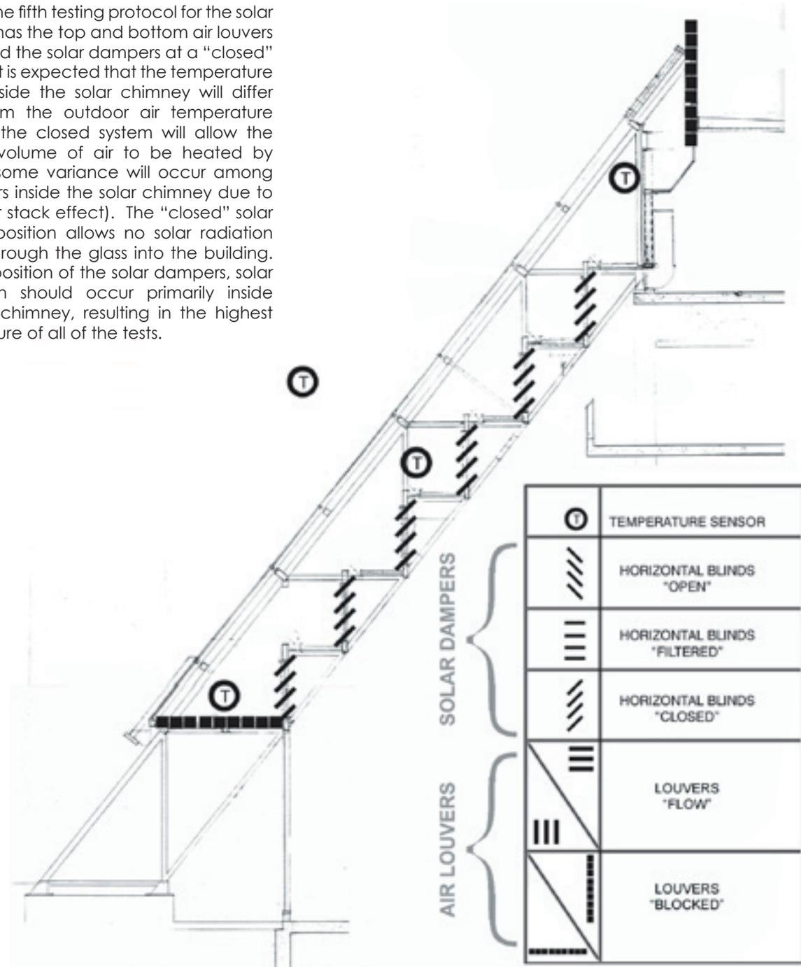
Figure 22.A. Test 5: Sunlight Closed/Air Blocked.
