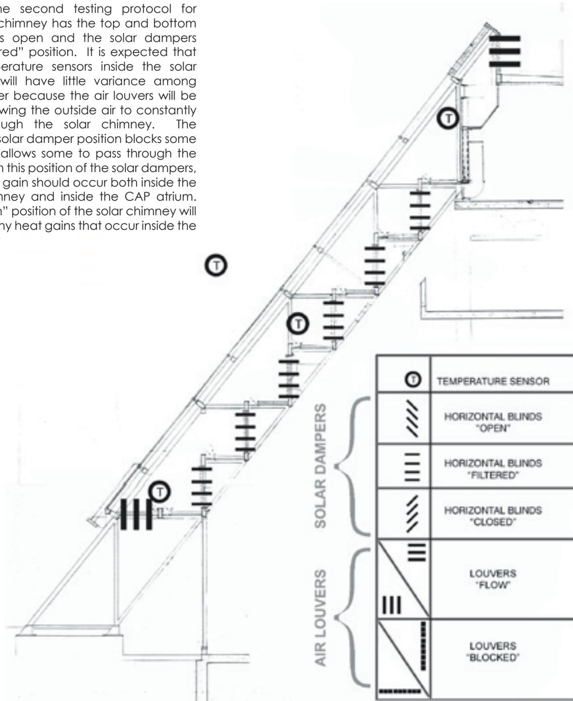
Figure 19.A. Test 2: Sunlight Filtered/Air Flow.
