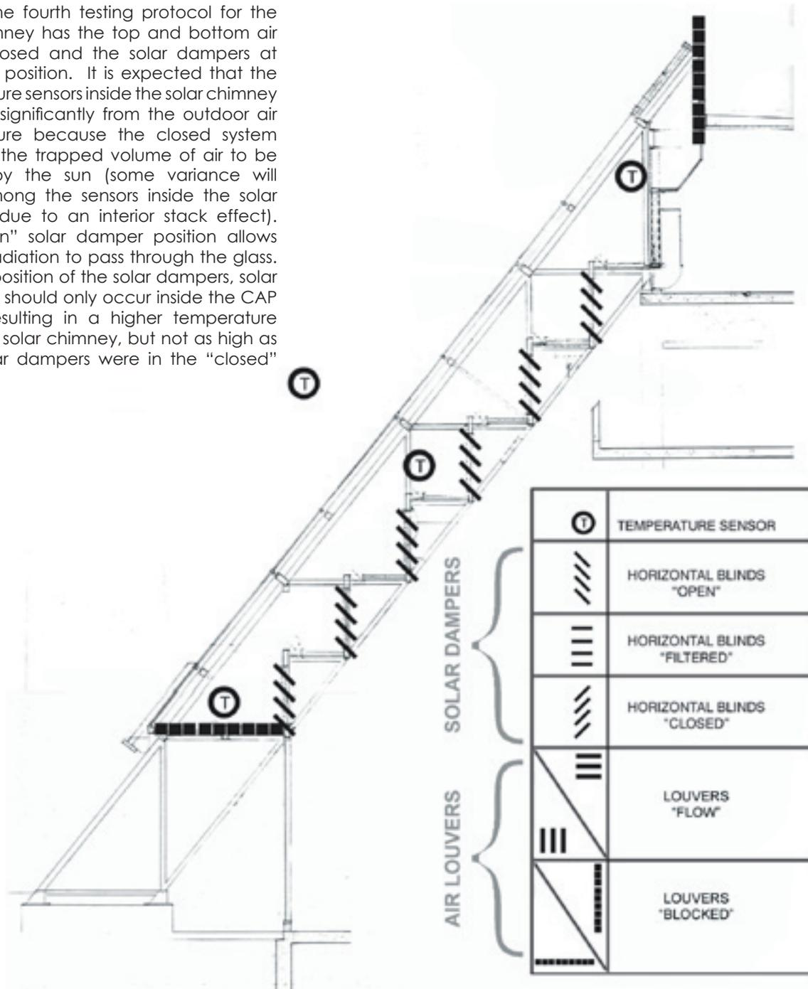
Figure 21.A. Test 4: Sunlight Open/Air Blocked.
