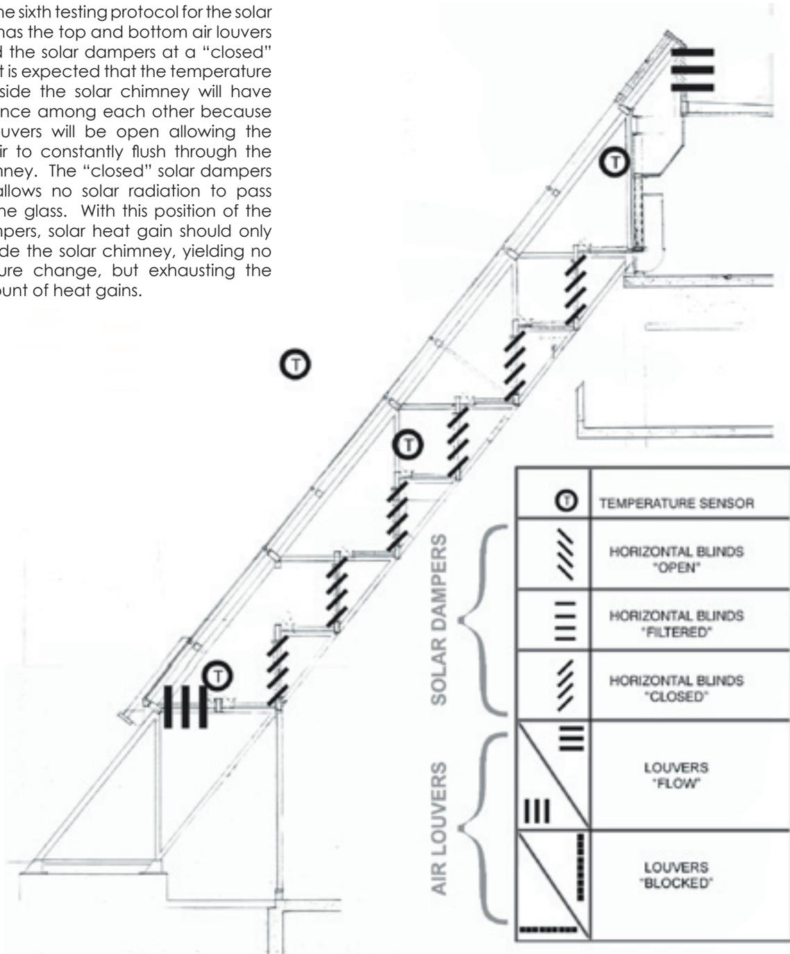
Figure 23.A. Test 6: Sunlight Closed/Air Flow.
