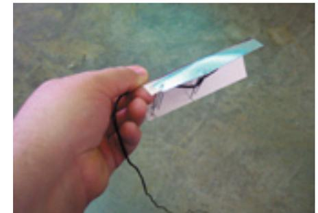
Figure 25.2. Detail of sun shield and wire sensor. (Photo by Robert J. Patton, 2003)
