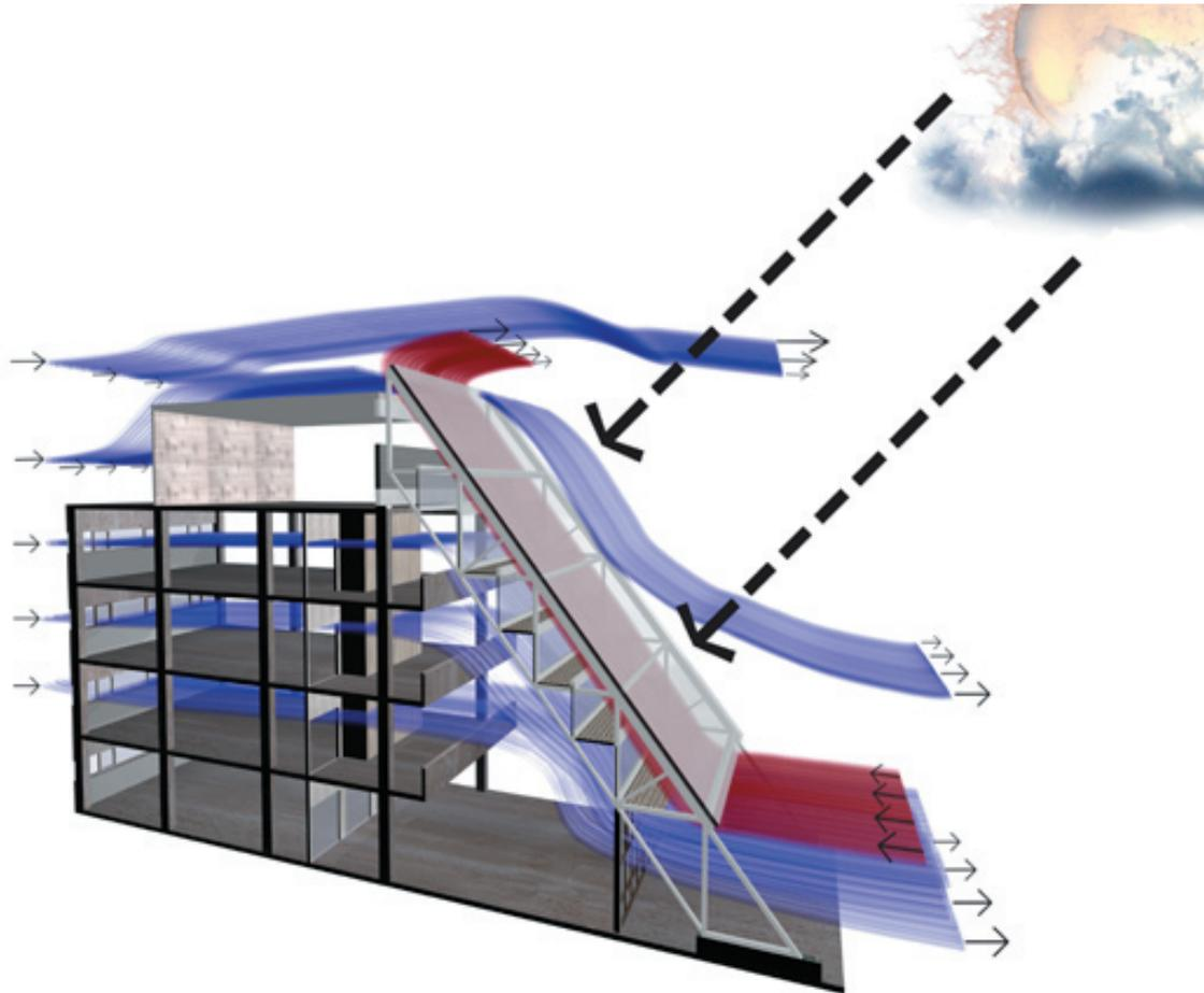
**Figure 17.A.** Natural Ventilation scheme B.
