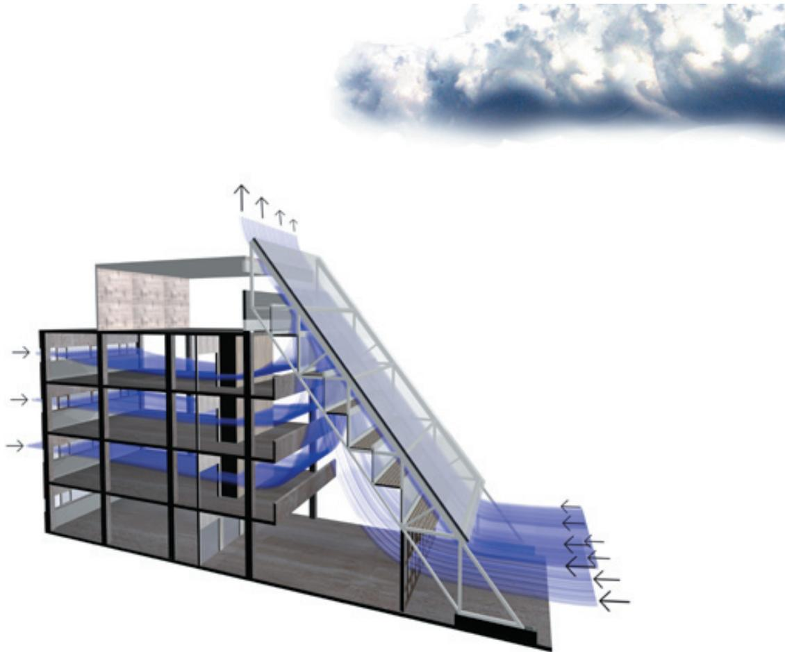
**Figure 15.A.** Natural Ventilation scheme D.
