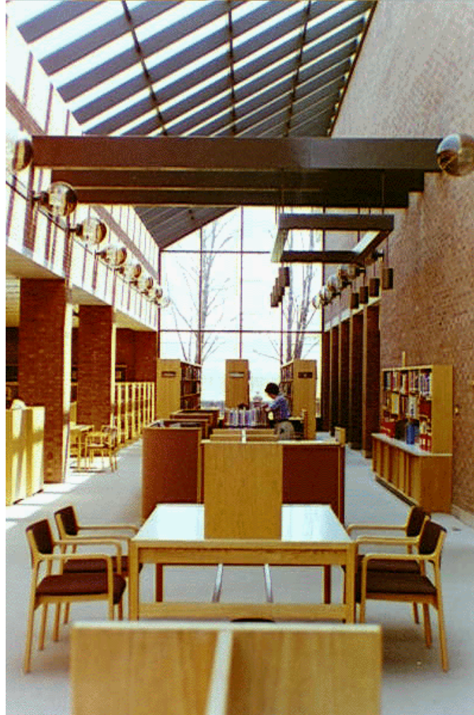
Figure 2 Interior view of galleria looking east, showing glazing system, and globe and track lighting fixtures.
