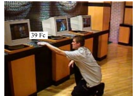
Figure 29.3 Instantaneous light measurement read 39Fc at 2'-6" above finished floor.
