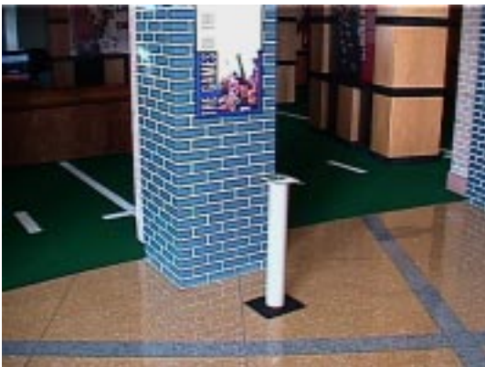
Figure 42.2 1. Stow-Away meter location 2'-0" outside gallery entrance, 30" AFF.
