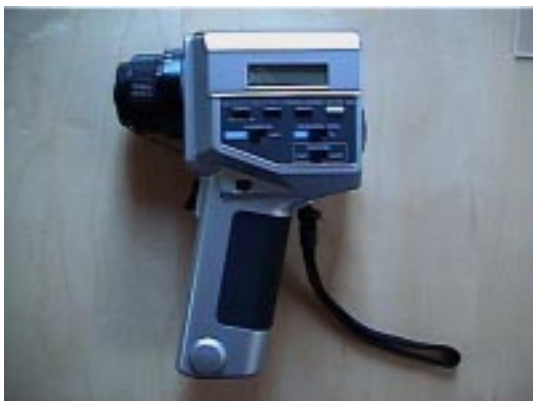
Figure 18.3 Data collection instrument: Minolta, LS-100 Direct-reading, narrow-angle spot-type luminance meter.
