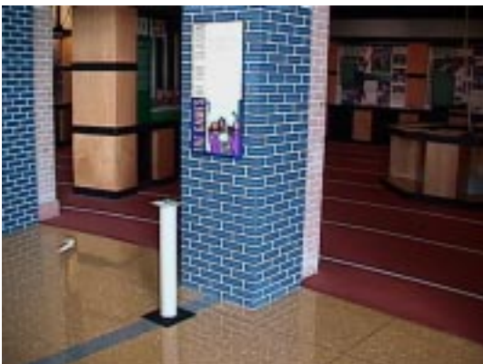
Figure 42.3 6. Stow-Away meter location 2'-0" outside gallery exit, 30" AFF.
