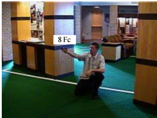
Figure 26.1 Collection of instantaneous spot illuminance. Readings taken in this manner to insure accuracy.
