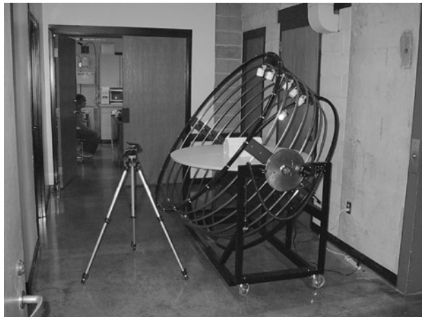
Image showing the heliodon, model placement, and tripod location
