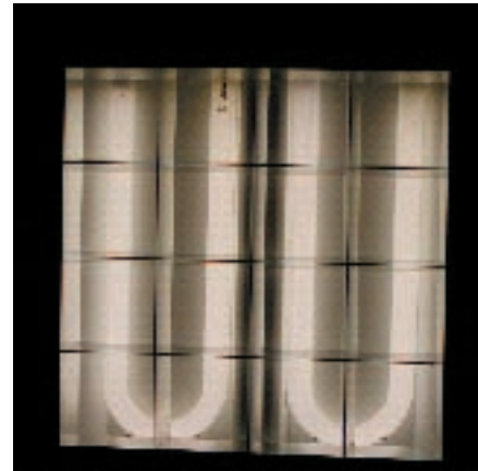
FIG. 3.1 34 W, T12 Curvalume rapid start SUPER SAVER fluorescent lamp, 6" leg spacing, Cool White phosphor, 4200K color temperature, 62 CRI ECO-LOGIC
