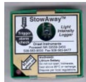
Fig. 15 Light intensity data logger used to take illuminance measurements over a two day period.
