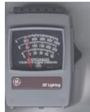
Fig. 14 GE handheld analog meter used to take instantaneous illuminance and luminance measurements.
