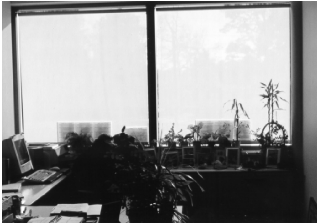
Figure 14: View from doorway showing contrast between office and exterior background when shades are pulled down all the way on a sunny afternoon. The details in the room are totally eliminated and some objects start to look as if they are one. Veiling glare occurs on these surfaces.
