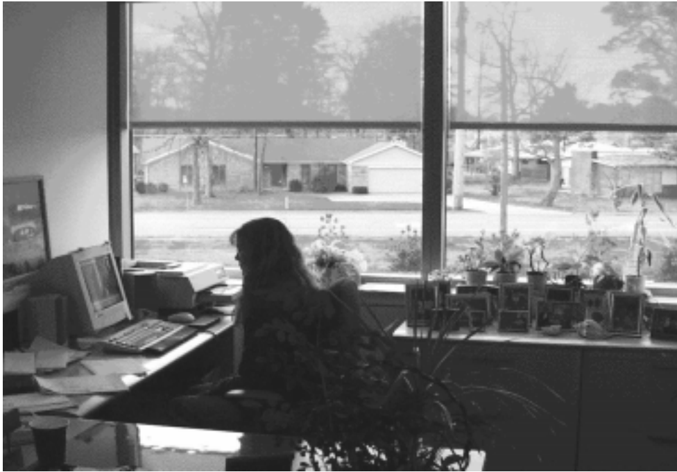
Figure 12: Scene from doorway of team member posing as occupant working at computer in heavily lit environment. Due to the brightness of the background, the details of the individual and other objects are lost from the view.
