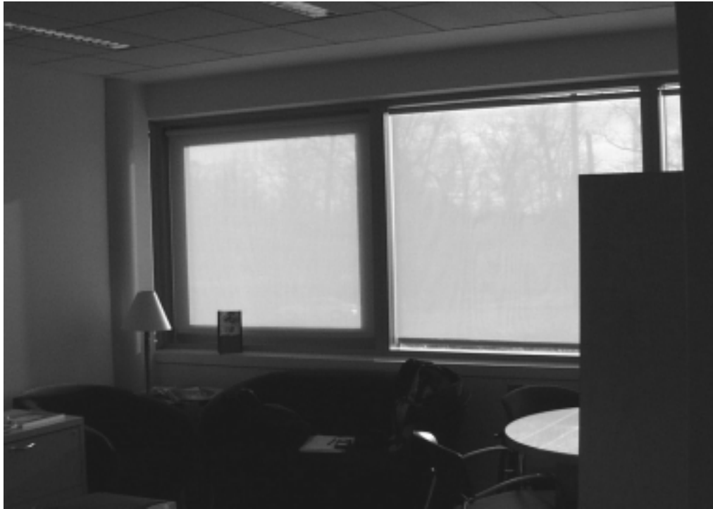
Figure 34: View of windows in office 256 as one enters the room on a sunny afternoon. Due to the room's arrangement as one enter they encounter veiling glare.
