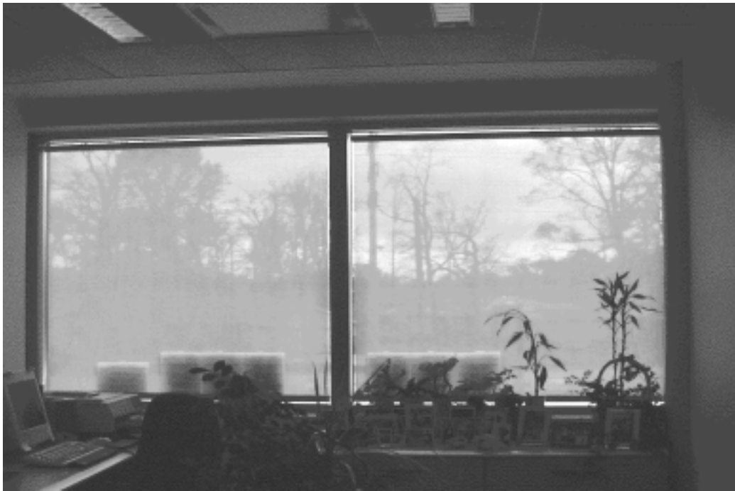
Figure 15: View of office 255 from doorway on an overcast afternoon. In these overcast conditions, it can be seen that the lack of reflection disables one's ability to distinguish objects from one another.
