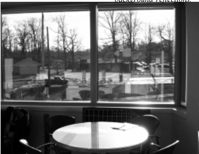
Figure 38: View of veiling reflections along with reflections in windows leading to unclear views.
